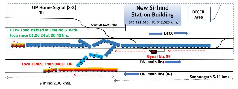
Collision & Derailment of loco no.33469/WAG9/CNB of Train no.04681 Exp between SIR-SDY on IR after SPAD of GVGN load, loco 60059/WAG-12/MELS at New Sirhind station (DFCCIL section) on 02.06.2024
